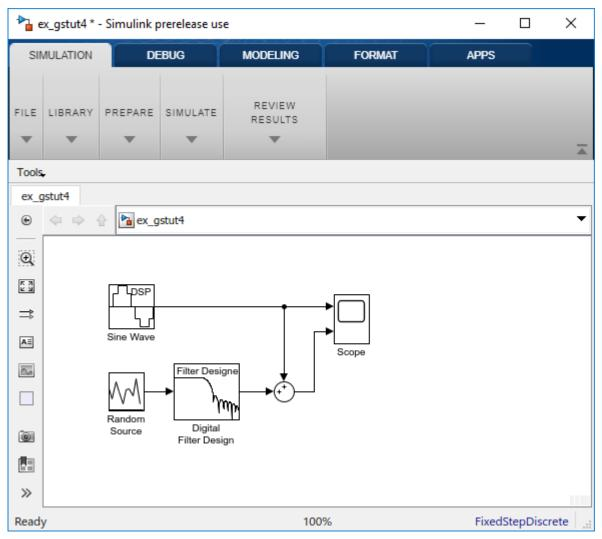
Run your model and view the results in the Scope window. This window shows the original input signal and the signal with low frequency noise added to it.
