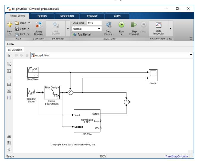
The positive input to the second Sum block is the sum of the input signal and the low frequency noise, s(n) + v. The negative input to the second Sum block is the LMS Filter block's best
